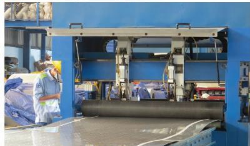
WWW.HOANGLAM Dimple welding
